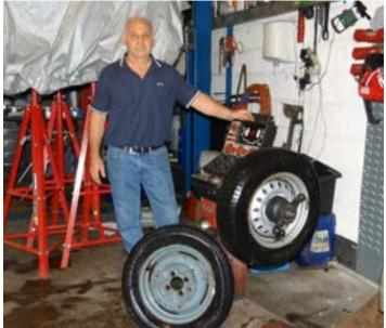
This new service has also involved acquiring his own balancing machine and making his own cones to fit the various classic wheels he is regularly asked to supply tyres for. The hand machined fittings mean that he can get the perfect balance for older wheels.
