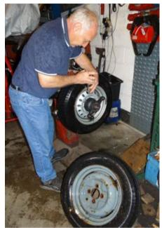
"The problem is that many of the modern tyre companies do not have the correct cones to fit classic wheels so the balancing is not as accurate as it should be," comments Darren.
